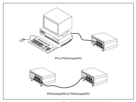
Figure 3-2. Basic MXI-3 Configurations
